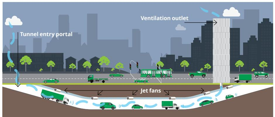
Traffic draws fresh air into tunnels at entry portals. Jet fans help move air along the tunnel towards the ventilation outlets. Ventilation outlets disperse emissions high into the atmosphere away from local communities.
